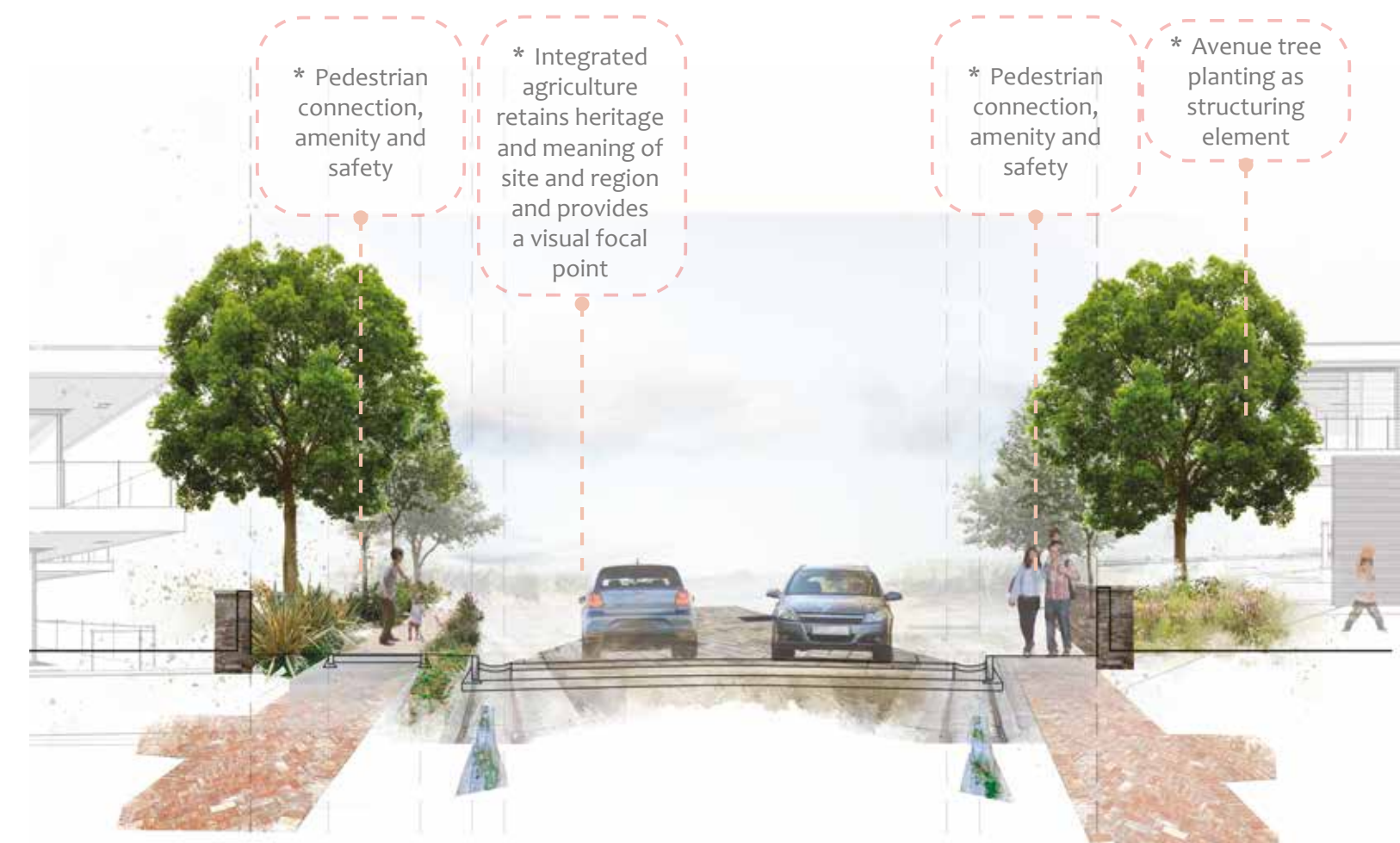
Fig. 32 Section 2 - Main Access Street against the contour
