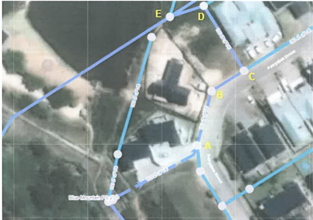
Figure 2: Upgrading of gravity sewers
